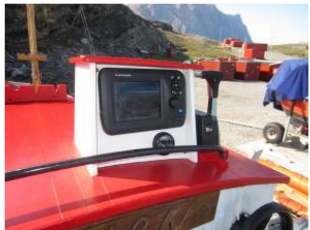
Left: The exhaust isolated with fire-retardant material. On the right the new bilge pump. Right: New GPS and temperature sensor installed in an instrument box made for the purpose.
