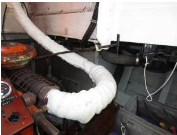
Left: The exhaust isolated with fire-retardant material. On the right the new bilge pump. Right: New GPS and temperature sensor installed in an instrument box made for the purpose.
