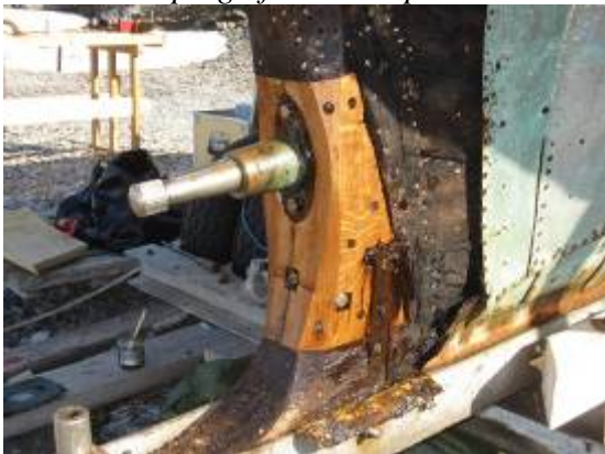
Reparation of the stern is completed
