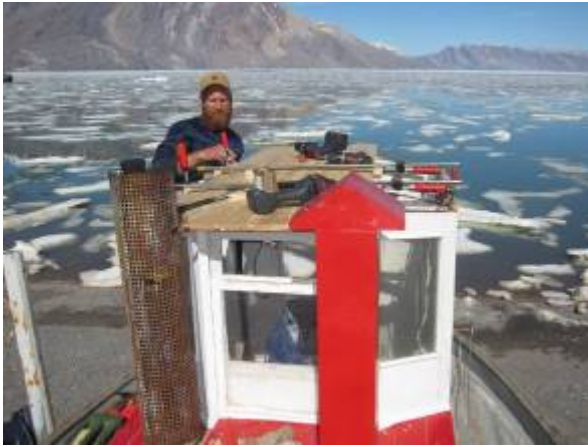
Left: Creation of a new wheelhouse roof. Right: The roof is finished and ready for painting.
