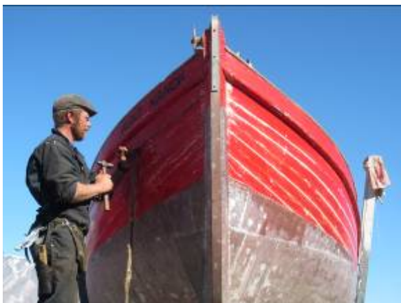
Left: Nicolai caulks the freeboard. Right: Caulking of the front of the deck.
